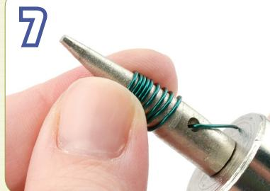
Work the wire up the cone mandrel, making sure the wire wraps side-by-side. Tighten your grip on the wire to create the best side-by-side wraps. Change the methods mentioned before to see if one creates tighter wraps for you.
