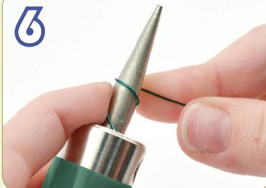
This step, similar to step 5 depends on personal preference. Try wrapping the wire around the mandrel with your dominant hand, or turn the mandrel and guide the wire onto the mandrel with your dominant hand. Switch these positions to find the method that you prefer.
