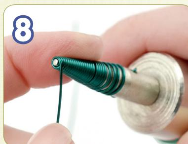
Take the wire to the very end of the mandrel, using caution when you release the wire as some unwinding will occur from the temper of the wire.
