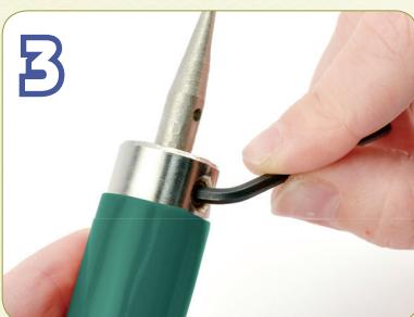
Tighten the allen screw with the wrench onto the flat portion of the shaft inserted into the holder.
