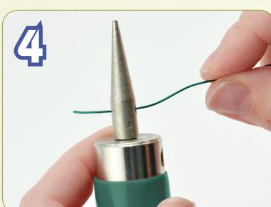
Insert one end of wire into the hole at the base of the cone mandrel. It's best to deposit the wire onto the mandrel before cutting the wire. General rule of thumb is about 18" (45 cm) of wire for the medium mandrel using 18 ga (1.0 mm) wire. You will need more wire for smaller gauges and less wire for larger gauges. Conestastic is made for 12 - 26 ga (2.1 - 0.41 mm) single wires.
