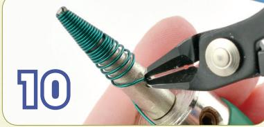
Cut the wire at the base to allow the cone to be free. Use this same cutting to adjust the length of the cone and trim the desired end with the flat side of the flush cutter against the wire end (as shown above in Step 9).
