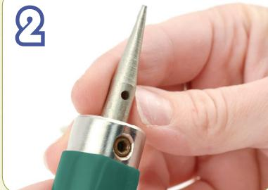
Insert chosen mandrel in the hole of the handle. Line up the flat side below the hole with the allen screw. This aligns the flat area on the shaft of the mandrel with the allen screw to assure no slippage of the mandrel and handle.
